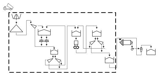
Figure 6. The focus of this is the crushing and screening stage in aggregate and mineral plants alike, depicted in the dashed box.
