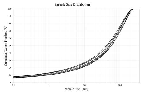
Figure 15. Variations of the particle size distribution for the incoming feed in a crushing plant simulation using the Swebrec function. The generated curves vary between 40-60 mm for  $x_{50}$  and 210-250 mm for  $x_{max}$ .
