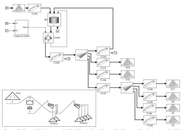
Figure 33. The modelled process in MATLAB/Simulink and the simplified layout of the plant in the embedded picture. The broad signal lines between the production units represent the material signal presented in Eq. 5.1 while the thin signal lines are process values  $(y_{pv}(t))$  and desired values  $(y_{sp}(t))$  explained in Eq. 5.11.
