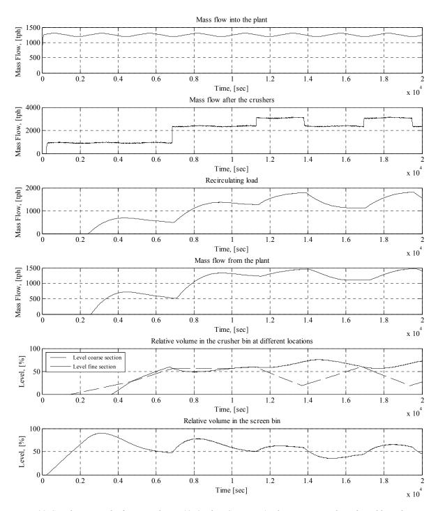
Figure 30. Simulation results from simulating 1250 tph in Scenario 1. The process is relatively stable with minor fluctuation.
