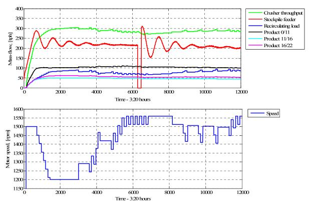
Figure 38. Simulation results after the optimization. The upper graph illustrates the mass-flow on different conveyors while the lower one illustrates the change in speed set point during the simulation.
