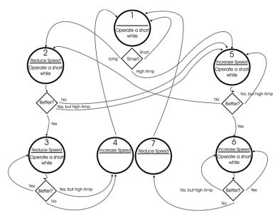
Figure 32. The FSM used for selecting appropriate speed [10].
