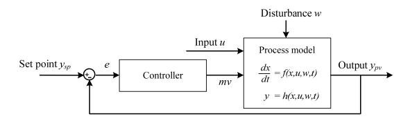
Figure 18. General representation of a feedback control loop. Modified from Marlin [51].
