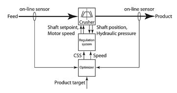
Figure 5. A closed loop process control for controlling the CSS and the eccentric speed of a cone crusher, as presented by Hulthén [10].
