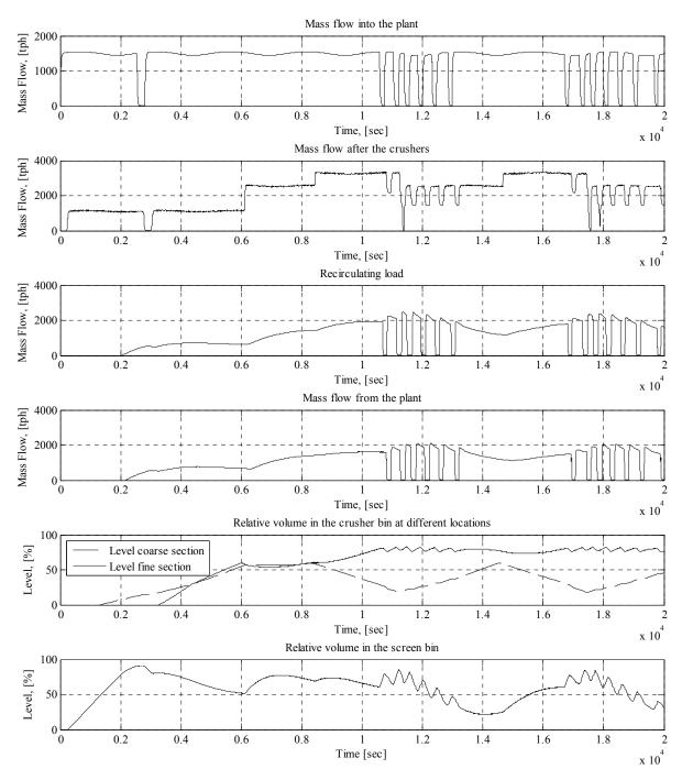
Figure 31: Simulation results from simulating 1500 tph in Scenario 1. The process starts experiencing major fluctuation after approximately 3 hours.
