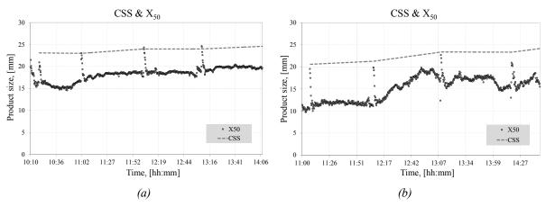
Figure 25 The trend of CSS (dotted grey line - interpolated between tests) and  $x_{50}$ , (black dots – calculated from logged process readings) as a function of material flow through the crusher at two of the experiments, (a) and (b). The results are close to parallel. Spikes in the  $x_{50}$  curve indicate an interruption in the process due to calibrations or mechanical failure.
