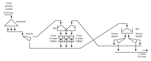
Figure 28. Flowsheet of the crushing section of the platinum processing plant as presented in Paper B.
