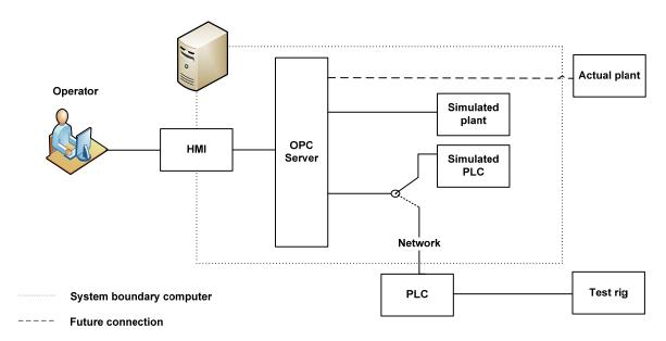
Figure 34. System architecture for enabling operator training.
