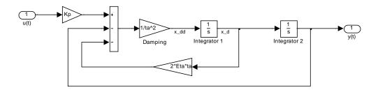
Figure 22. Representation of Eq. 5.14, the second order system without delay as a differential equation in MATLAB/Simulink.
