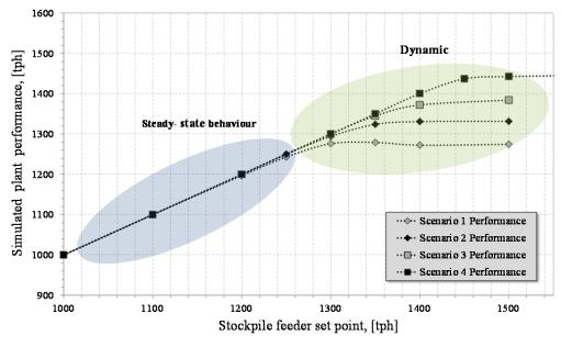
Figure 40. Plant's average production performance. In the blue area the plant operates in steady-state while in the green area the plant experiences fluctuation and limited throughput.
