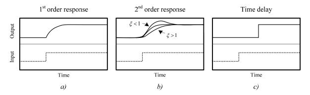
Figure 20. Step response for first order system (a), second order system (b) and a pure time delay (c). Modified from Marlin [51].
