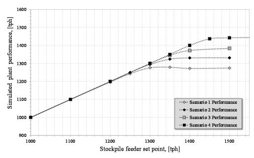
Figure 35. Average plant performance for different feed rates and plant configuration.
