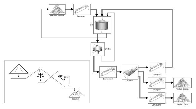
Figure 11. Flowsheet of a single crushing state in MATLAB/Simulink with a simplified layout of the plant in the embedded picture. The broad signal lines between the production units represent the material signal presented in Eq. 5.1 while the thin signal lines are process values  $(y_{pv}(t))$  explained in Eq. 5.11.
