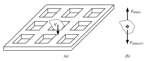
Figure 3. Two methods of separating the material with respect to certain particle size. With a fixed aperture (a) and with relative drag force (b).
