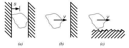
Figure 2. Schematic principles of form conditioned crushing (a), energy conditioned crushing (b) and attrition (c), as presented by Evertsson [5].
