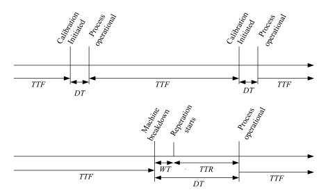
Figure 16. Two different example scenarios for discrete events. The scenario above illustrates the calibration process as an event while the scenario below illustrates the consequence of machine breakdown.
