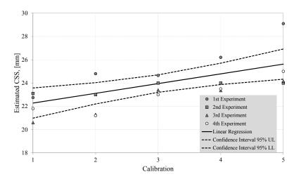
Figure 26 Wear trend (black line) generated from the results of the calibration with a calculated 95% confidence interval (black dotted lines).
