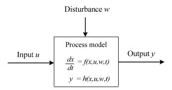
Figure 12. General representation of a dynamic system. The output y and dx/dt are functions of the input u, the disturbance w and the internal variable x, with respect to time t.
