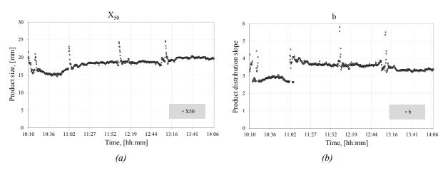
Figure 24. Calculating the change in the particle size distribution,  $x_{50}$  (a) and b (b), over time from the logged process reading.
