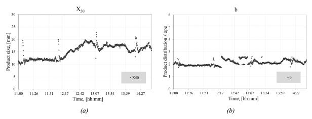
Figure 23. Calculating the change in the particle size distribution,  $x_{50}$  (a) and b (b), over time from the logged process readings.
