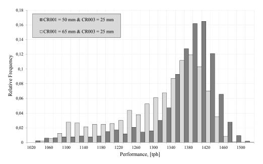
Figure 36. Plant performance for two different settings of crusher 1 (CR001).
