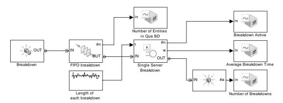
Figure 17. Event generated with SimEvents for representing a mechanical breakdown.
