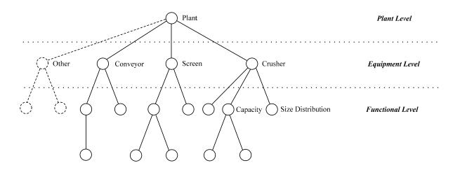
Figure 10. Illustration of the system hierarchy.
