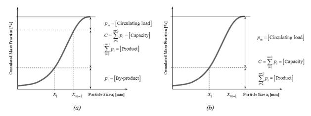
Figure 4. Schematic illustration of capacity, product, circulating load and by-product identified on a particle size distribution for aggregate (a) respectively mining application (b), as presented by Lee [6].
