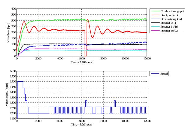
Figure 37. Simulation results with existing settings. The upper graph illustrates the mass-flow on different conveyors while the lower one illustrates the change in speed set point during the simulation.
