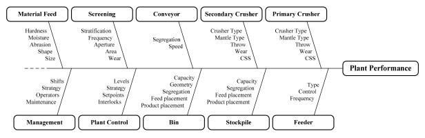
Figure 9. Cause-and-effect diagram over factors that can influence plant performance.
